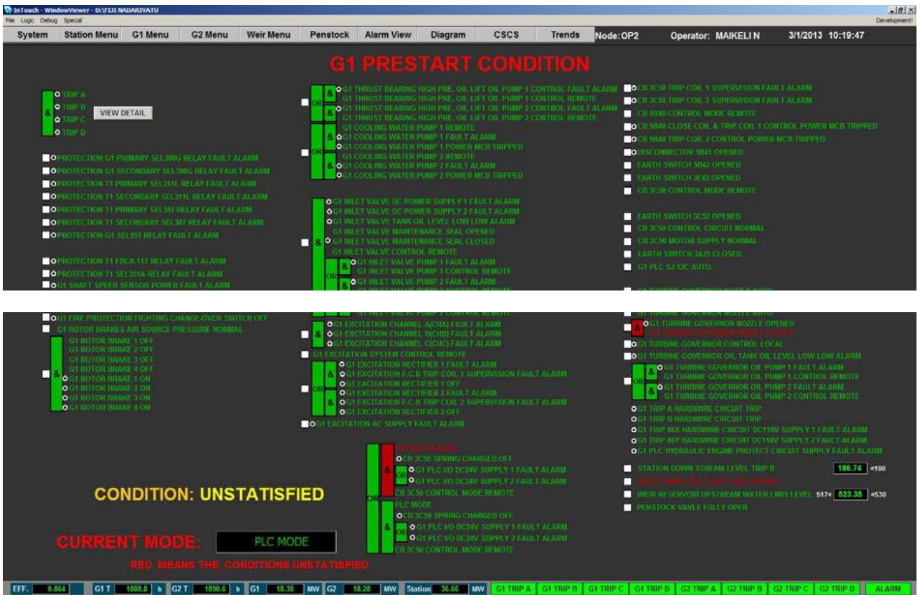
Figure 9-12: Unit Prestart Conditions
