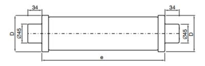
Figure 1: shows the dimensions of the ABB circuit breaker fuse
