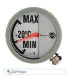
The movement of the float is normally radial to the casing. The "G" version is recommended for installation in narrow or flat conservators in which only limited movement is possible; in this case the float movement is axial to the casing and the display can be scaled at a ratio of 1:1, 1:2, 1:3 or 1:4.
