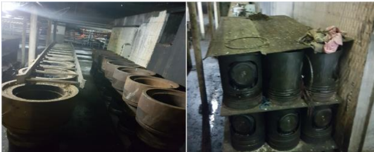
Figure 2: basement scrap 2: cylinder liners and pistons
