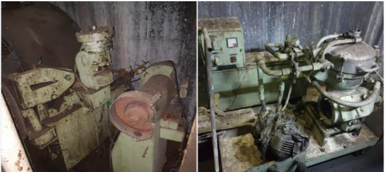
Figure 4: basement scrap 4: 3 phase grinder and 3 phase centrifuge
