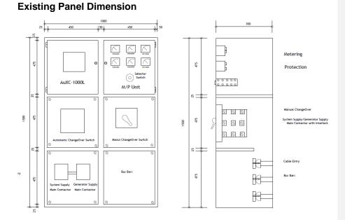
**Note**; The above drawing gives the exact existing panel dimension but the design is not as per on site. Length 1000mm, width 300mm and height is 1500mm. The above design is something for the Bidder to consider on their design.
