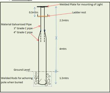
The poles should be rust treated and painted in silver metallic paint and also have provision for earthing connection of the same.
